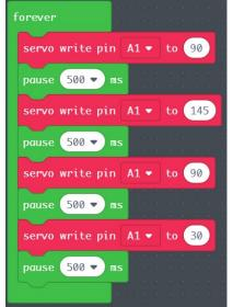
A continuous rotation servo acts like a motor. A value of 90 stops the servo. Values between 0 and 85 rotate the shaft backwards, and between 95 and 180 rotate the shaft forwards.
