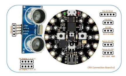
The ultrasonic sensor requires a signal (A6) to trigger a sound wave and a signal when the echo is received back (A7).
