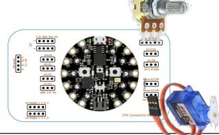
Change the potentiometer with the soil moisture sensor, and use it to control the servo. Try both types of servo.
