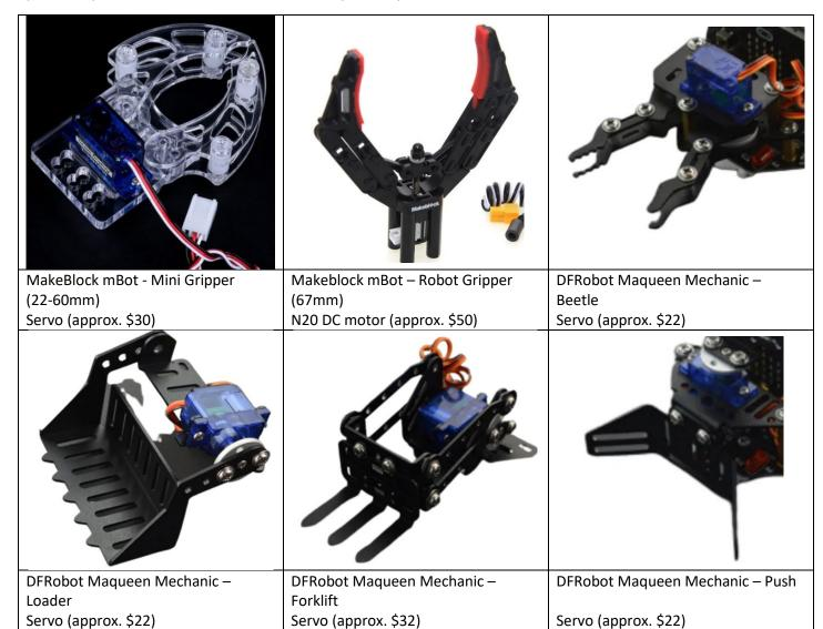
These are all easily mounted on the mBot2 by adding a wooden or metal bar in front of the ultrasonic sensor (which may need raising slightly).
