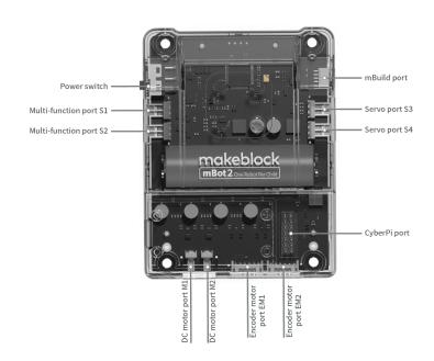
The Power Switch must be turned on before the you can upload code
