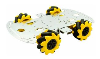
These wheels can be driven using the EM motor outputs combined with motor outputs M1 and M2.
